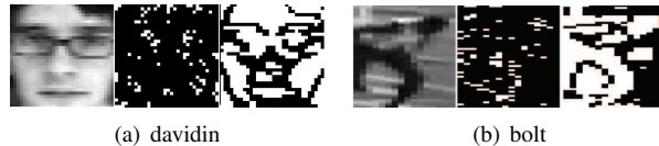
Figure 2. Comparison of two feature selection methods based on different loss functions. A white pixel indicates that the corresponding feature is selected, otherwise black. For each of the two sequences, the original image, the LASSO result and the sparse regularized logistic regression result are shown from left to right.
